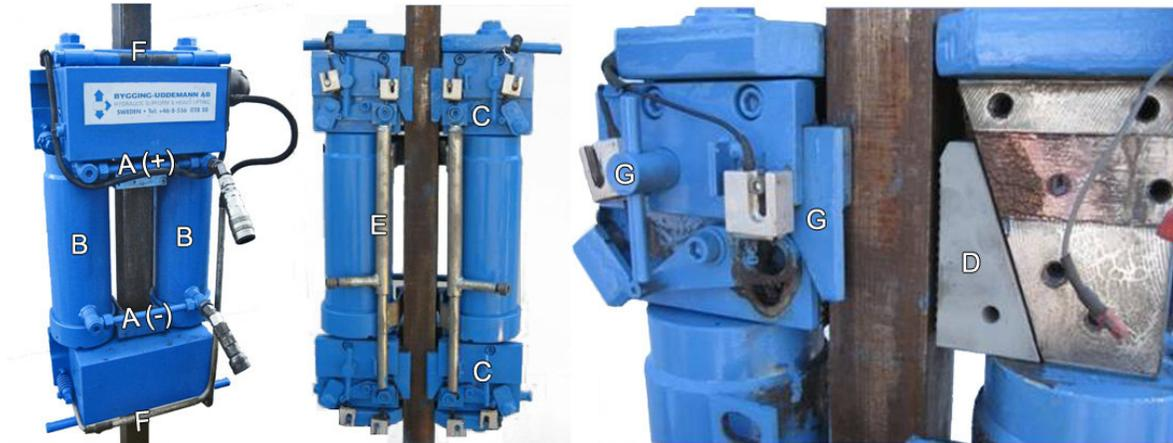
*Fig. 1. (A) Branch pipe, (B) Hydraulic cylinders, (C) Grip jaw head, (D) Grip jaws, (E) Switch mechanism, (F) Top-bottom plate, (G) Catches with Operating shafts.*
